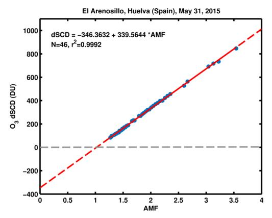
**Figure 2.** Langley extrapolation applied to the dSCDs derived from Phaethon measurements on May 31, 2015. The constant term of the linear regression gives the -SCD<sub>REF</sub>, while the slope corresponds to the mean VCD of the reference day.
