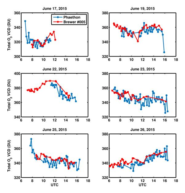
**Figure 7.** Total  $O_3$  VCD obtained from both the Phaethon system and Brewer #005 at LAP in Thessaloniki after the campaign period.
