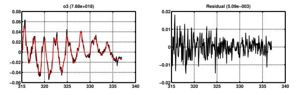
**Figure 1.** Example of differential slant column fit for  $O_3$  obtained with Phaethon from direct sun irradiance measurements at SZA=58° (May 31, 2015). The left panel shows the measured (black) and the fitted (red) values, and the right panel shows the residual from the DOAS fit.
