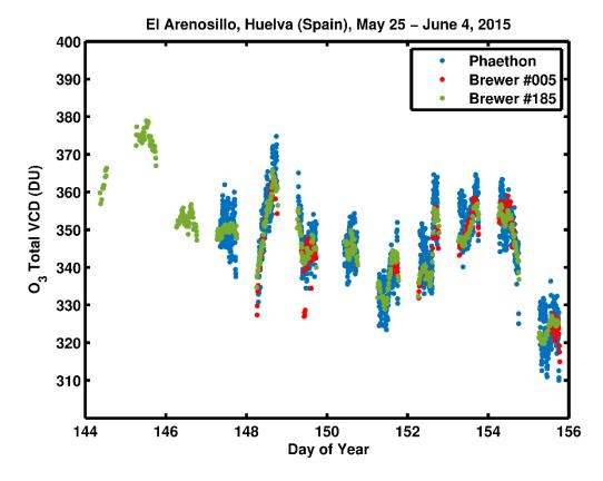
**Figure 4.** Total  $O_3$  VCD time series obtained from Phaethon system during the campaign. Brewer #005 and #185 measurements are also presented.
