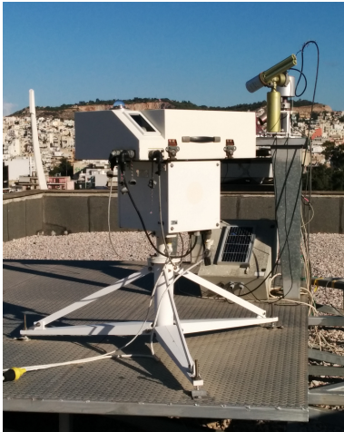
Figure 1: The MKIV Brewer #001 spectrophotometer and the Cimel sun/sky photometer on the roof of the Biomedical Research Foundation.
