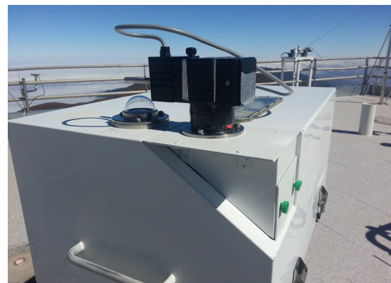
Figure 1. UVB Dome, direct port looking to the zenith and direct port looking normal to the window.
