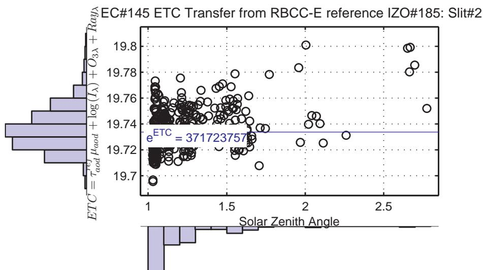
Figure 11: Brewer #145 calibration factor transfer for wavelength 310.1 nm using Brewer #185 as a reference.
