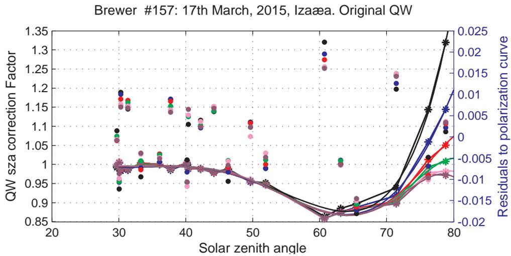
(a) SZA dependence for Brewer #157. The solid curves are 6-degree polynomial fits on the data, whereas the dots are residuals to the fitting curves. Measurements were performed using the original QW.
