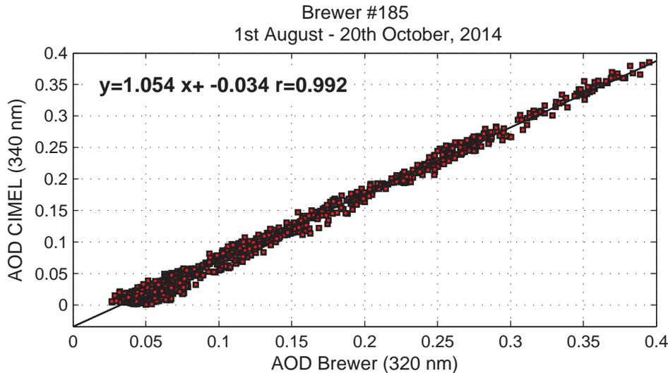
Figure 9: Scatterplot of instantaneous Cimel (wavelength 340 nm) and Brewer (wavelength 320 nm) AOD data. The data were selected to be within a 5 min window.
