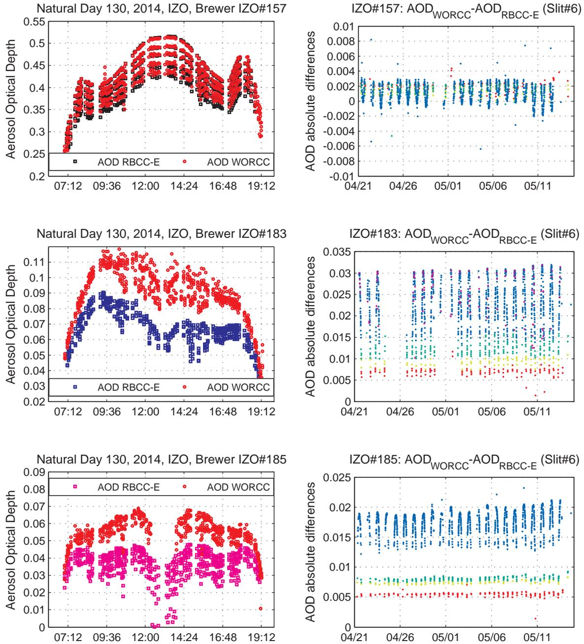
Figure 2: Aerosol optical depth (left panel) calculated independently for RBCC-E Brewer Triad using two different algorithms: WORCC (red circles) and RBCC-E (color squares). We show in the right panel AOD deviations (absolute differences grouped by Brewer neutral density filters) between both algorithms during the period from 21th April to 15th May, 2014.
