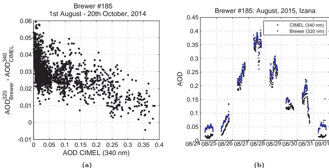
Figure 10: Differences between Brewer and Cimel data sets as a function of the AOD measured by the Cimel (10(a)) and AOD data from both instruments during the period from 24th to 31th August, 2014 (10(b)).
