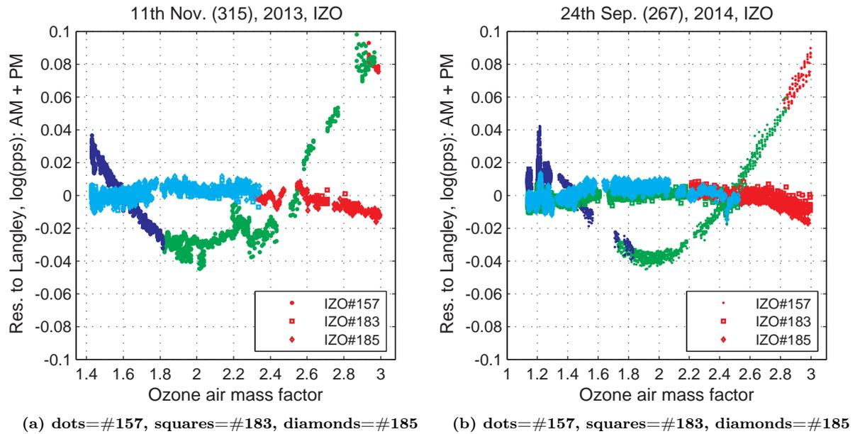
Figure 4: Residuals to Langley plot, grouped by Brewer neutral density filters, for RBCC-E Brewer Triad and for day 24th September, 2014 (natural day 267). Residuals are calculated in logarithm scale, that is,  $\log(I) - RegressionLine_{Langley}$ .
