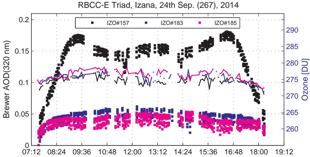
Figure 3: Aerosol optical depth at 5 wavelengths (306.3, 310.1, 313.5, 316.8 and 320.1 nm, color squares) and ozone (color solid lines) calculated for RBCC-E Brewer Triad using the RBCC-E algorithm for day 24th September, 2014 (natural day 267).
