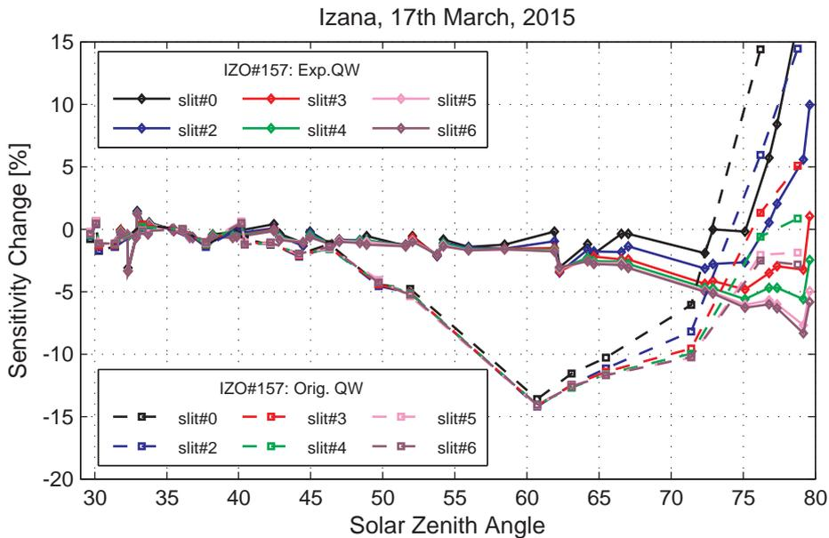
Figure 7: Change in Brewer #157 sensitivity as a function of SZA from field measurements at 5 wavelengths (306.3, 310.1, 313.5, 316.8 and 320.1nm) with and without the QW. Different data sets correspond to the experimental QW (solid lines) and the original QW (dashed lines). The derived changes are normalized to  $SZA = 35^\circ$ .
