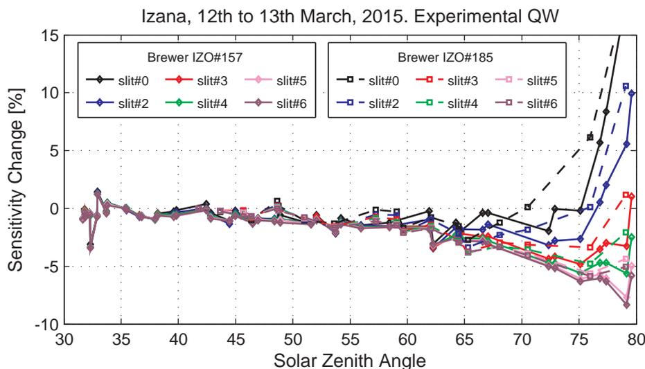
Figure 5: Change in Brewer #157 (solid lines) and #185 (dashed lines) sensitivity as a function of SZA from field measurements at 5 wavelengths (306.3, 310.1, 313.5, 316.8 and 320.1nm) with and without the experimental QW. The derived changes are normalized to  $SZA = 35^\circ$  for Brewer #157 and to  $SZA = 42^\circ$  for Brewer #185.
