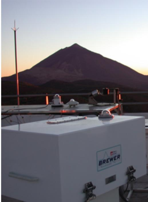
Figure 1: The Regional Brewer Calibration Centre-Europe (RBCC-E) traveling standard Brewer #185 at the Izaña Observatory.
